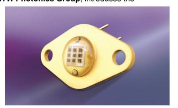
Opto Diode's new device provides an exceptionally uniform optical beam. The spectral bandwidth at 50% is typically 40 nm, and the half-intensity beam angle is 120 degrees. All surfaces on the standard 2-lead, TO-66 electrically-isolated package are gold plate.
